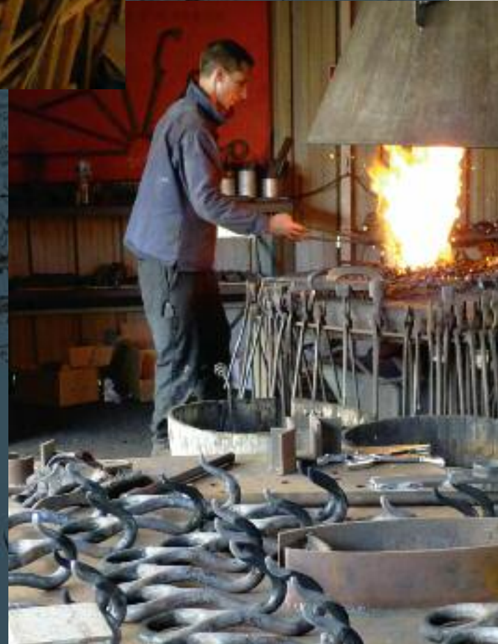
A blacksmith's forge was installed at the Arsenal specifically for the Hermione project. At work in the forge, this ironmonger uses traditional techniques to produce hardware to be used as part of the rigging.
