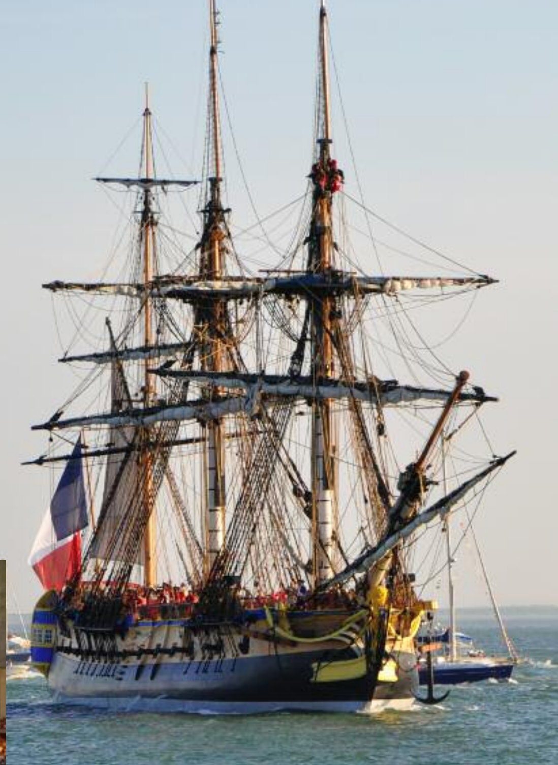
Sea trials were conducted between September and November of 2014. Sea trials determine if a vessel is seaworthy and are an important final step in the construction process. Hermione sailed along the west coast of France between Brittany and Bordeaux.
