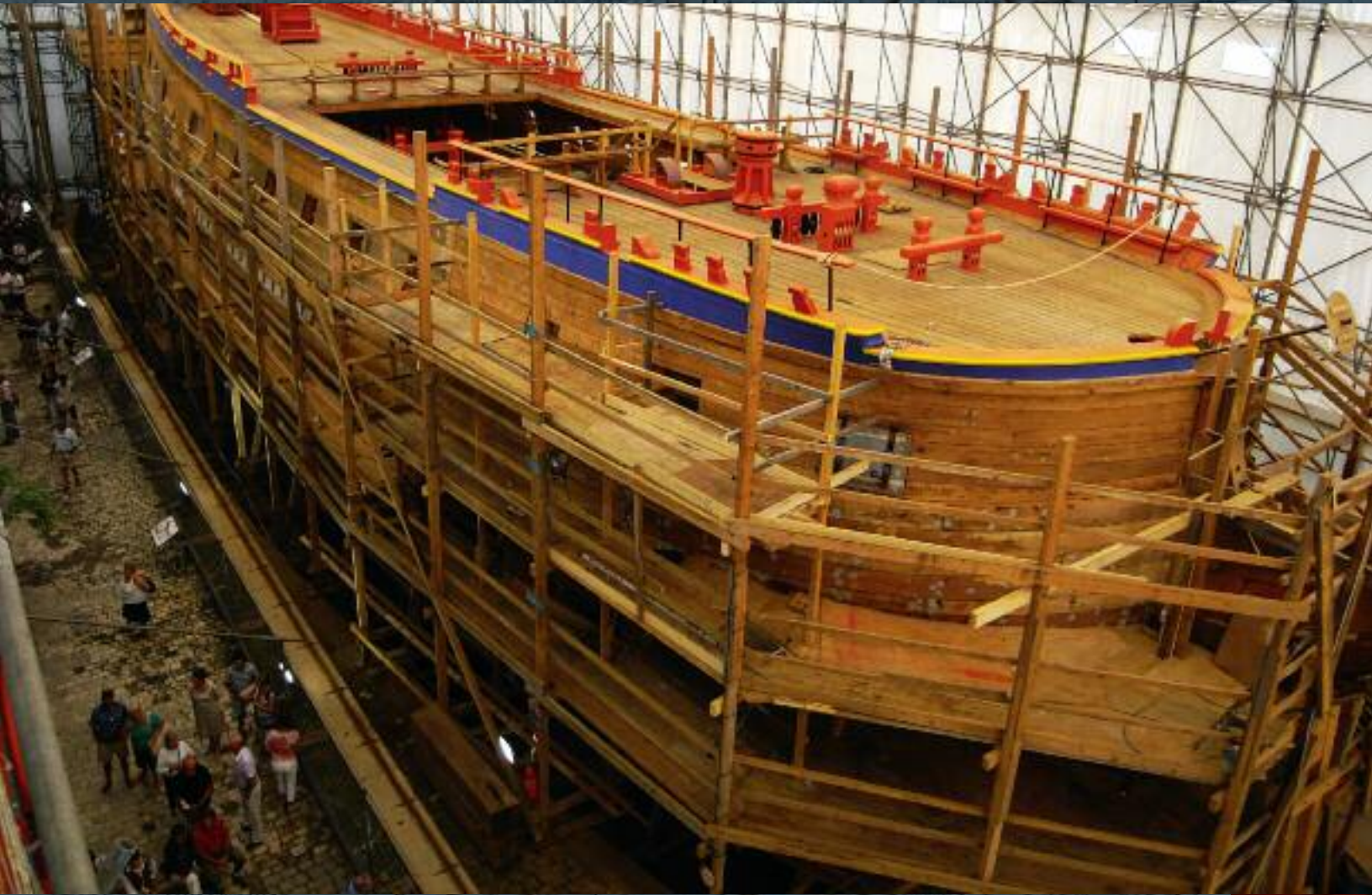
A view from 2009 of the Hermione under construction in drydock at Rochefort. Similar to the engraving from the Art de Batir les Vaisseaux , here the construction crew has built wooden scaffolding for the ship. The vessel was built from the ground up. Once the keel was laid, the hull and decks were finished before attention turned to the masts and rigging.
